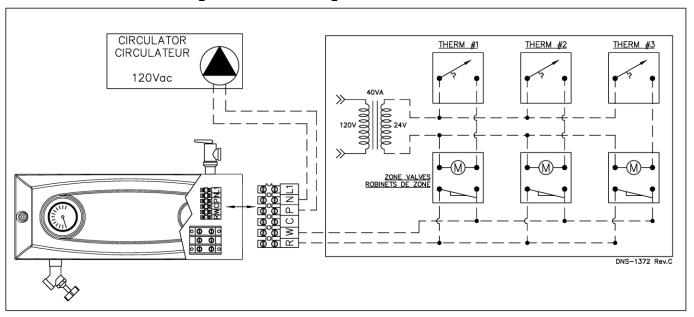
Figure 7: Electrical Diagram
