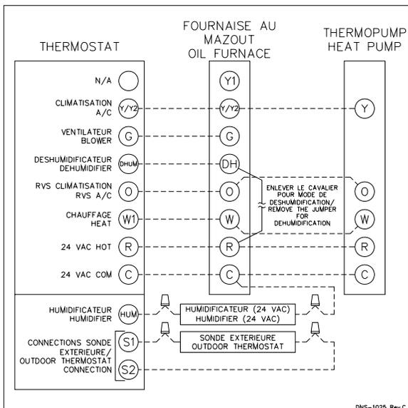
Note: On units with 2 stage cooling or heat pump, terminal Y1
